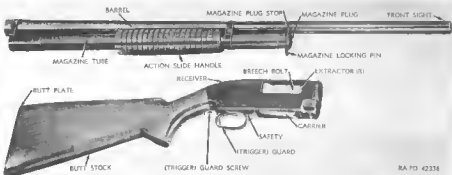
Figure 27—Gun Taken Down—Right Side View—Showing Location of Parts— Winchester Shotgun M12 (Take-down)
